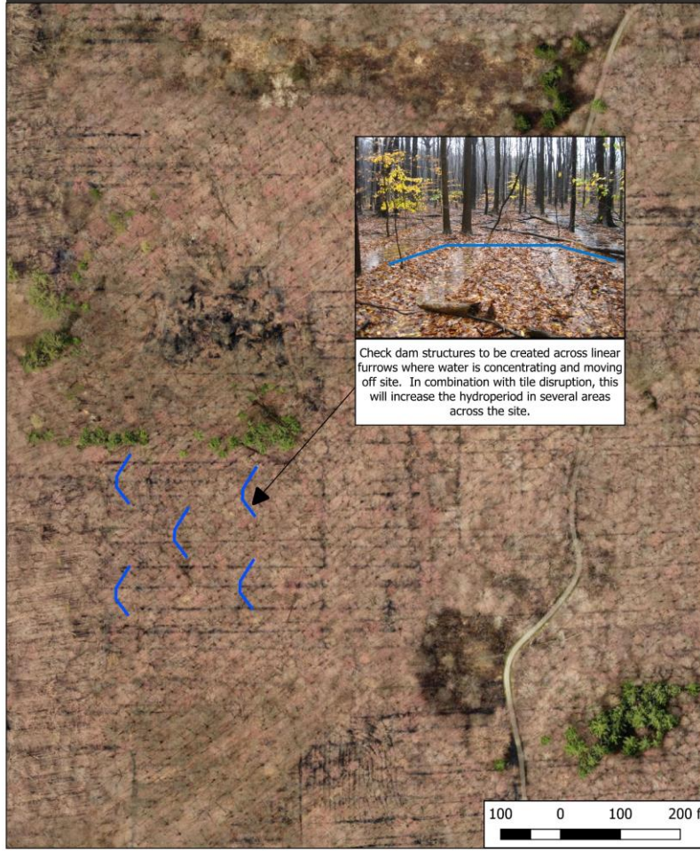
S.O.M Center Wetland Enhancement Site Hydrologic Enhancements - Check dams
